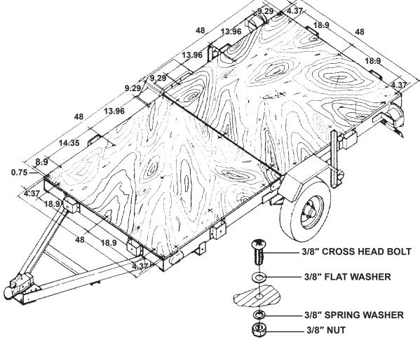
Figure L: Optional Bed Installation
